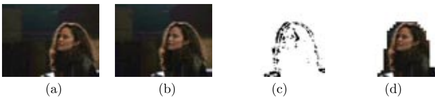
Figure 15: Key Object Segmentation Result in a shot of ‘ATF (action movie)’ (a) Frame #1948 (b) Frame #1949 (c) Difference Image (d) Segmentation Result
