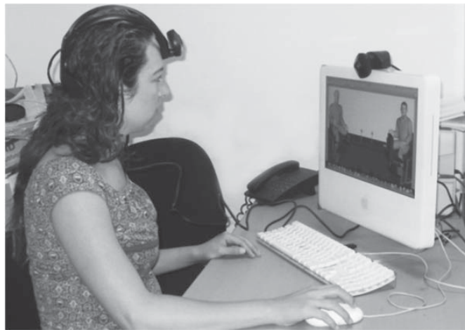
Figure. 1. A desktop virtual environment with head tracker
