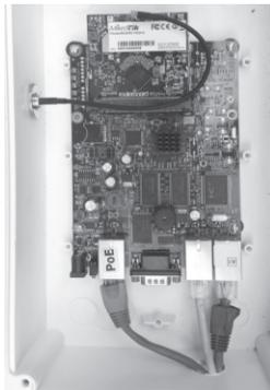
**Fig.14.** RouterBoard Rb433.
